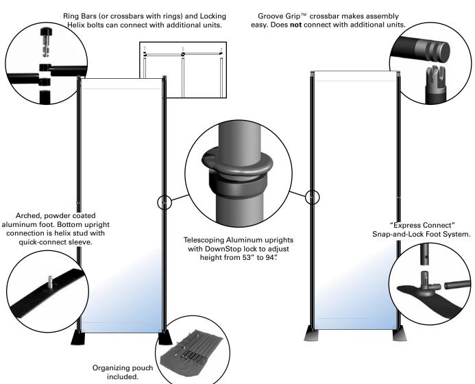
Our basic Core Unit is the starting point for many other configurations. This simple, one-panel display is available in varying widths from 20" to 120" and adjusts from 53" to 94" high. Panels and accessories can be swiftly assembled, changed, taken apart and packaged for easy and convenient travel from one presentation to another.
